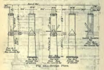
The old masonry was built up of concrete to the finish for 7-ft. deck plate girders, using vertical faces and not exceeding the size of the old piers. The length of this top section on the old masonry was 14 ft. on each of the piers, and the design of the new piers was similar in size and shape to the old mid-pier with its new top section.
